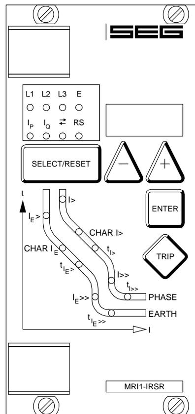
Figure 3.13: Front panel MRI1-IRSR; MRI1-IRE/IRX and MRI1-ISR
