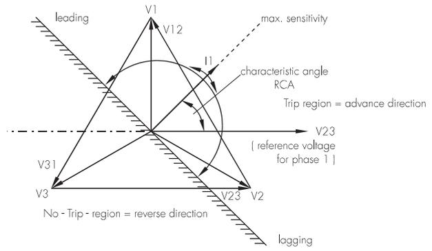
Figure 4.3: TRIP/NO-TRIP region for directional element in MR11. In this case the advance direction is defined as TRIP region and the reverse direction as NO-TRIP region.
