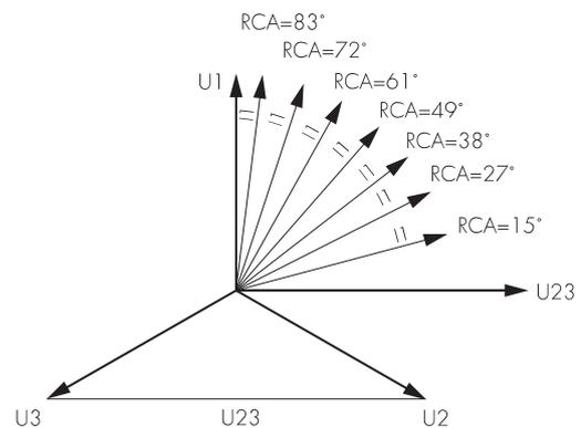
Figure 4.2: Relay characteristic angle
