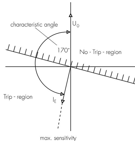
Figure 4.9: Characteristic angle in resistance-earthed systems (RESI)
