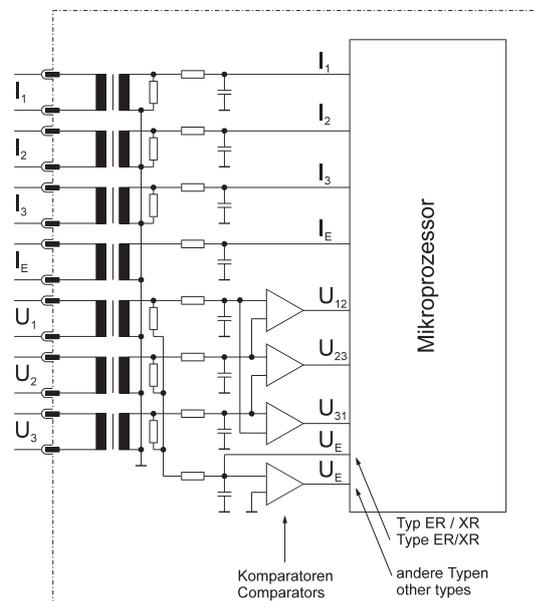
Figure 4.1: Block diagram
