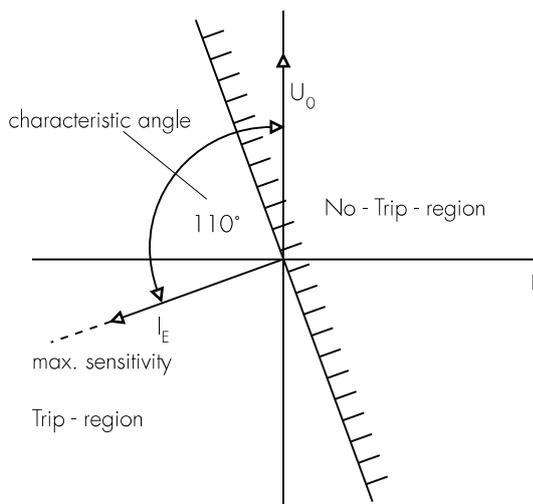
Figure 4.8: Characteristic angle in solidly earthed-systems (SOLI)
