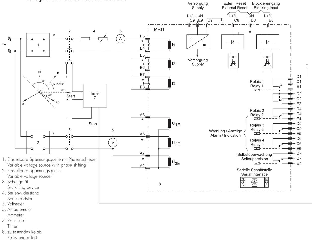
Figure 6.2: Test circuit
