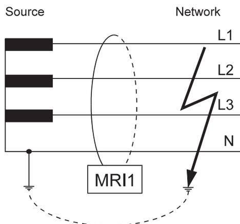
Figure 4.5: System earth fault protection
