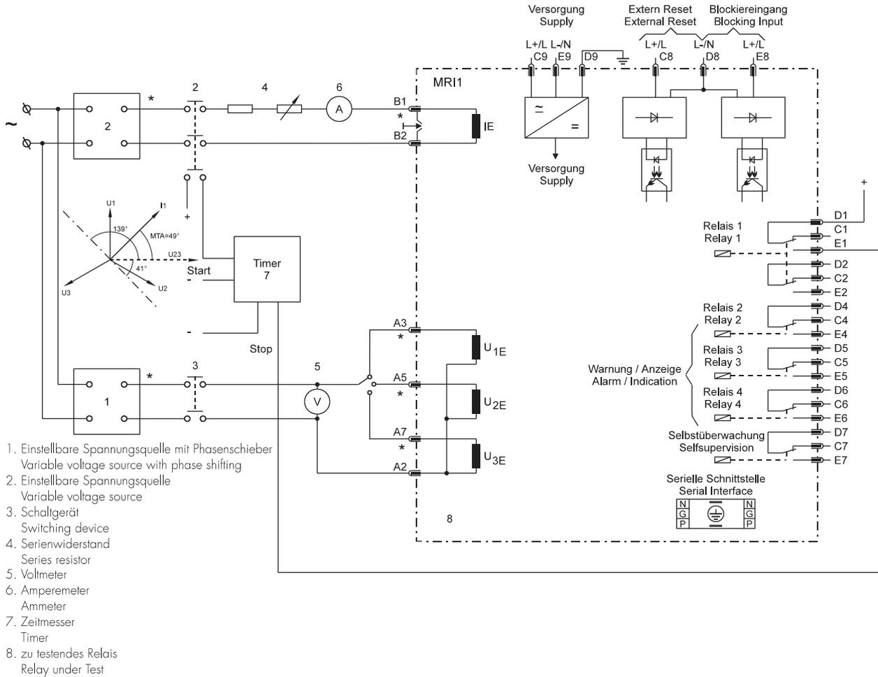
Figure 6.3: Test circuit
