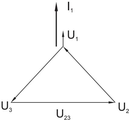
If line impedance and internal resistance of the generator is only inductive:
